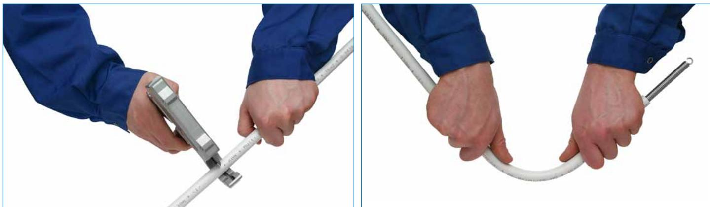
1. Cut a pipe at the right angle to its axis to a required length using scissors for multi-layer pipes or with a disc cutter.
