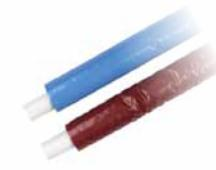
**KAN-therm** multilayer pipe PE-RT/AI/PE-HD Multi Universal designed for central heating, hot and cold water systems as well as for underfloor heating systems; operating pressure max. 10 bar
