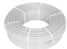
**KAN-therm** multilayer pipe PE-RT/AI/PE-RT Multi Universal designed for central heating, hot and cold water systems as well as for underfloor heating systems; operating pressure max. 10 bar - in 6 mm thermal insulation
