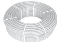
**KAN-therm** multilayer pipe PE-RT/AI/PE-RT Multi Universal designed for central heating, hot and cold water systems as well as for underfloor heating systems; operating pressure max. 10 bar
