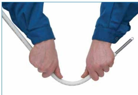
Shape the pipe as required. Bend using external or internal spring. Obey minimum bending radius  $R \geq 5$  Dz.
