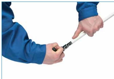
Calibrate the pipe and chamfer its internal edge with a calibrator but not deeper than down to the aluminium layer.
