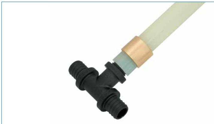
3. Expand the pipe with a hand or electric expanding tool. In both cases use the expanding tool in three stages. First two expansions not full, then rotate the expanding tool through 30° and 15° against the pipe. The third expansion is full.
