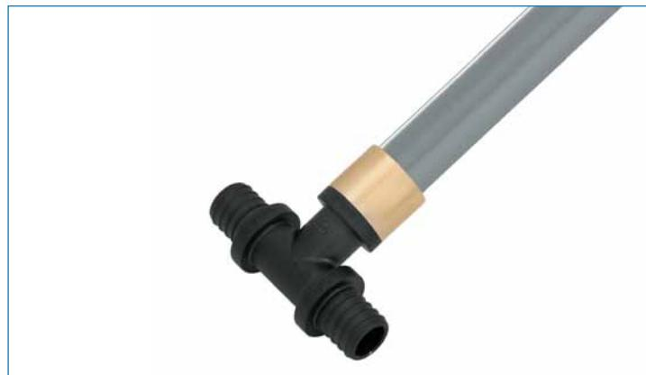
5. Slide the ring with a hand/hydraulic or electric machine Grip fittings only at their flange. Do not slide two rings at the same time.
