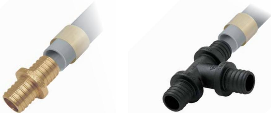
Push Platinum System leak-tight joints without O-rings are made by pushing a brass ring onto a fitting and a pipe. These connections do not require additional sealing like a PTFE tape or tow. The system is complemented by manifolds and installation cabinets available in section Manifolds, cabinets and accessories.
