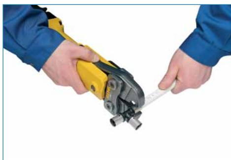
Apply the clamping tool jaws on a ring so it contacts the tube coupling collar. The external collar of jaws shall be pushed to the tube coupling collar but not embrace it.
