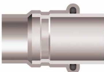
**Pic. 5** Press conection before and after press
