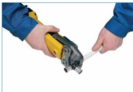
Start the clamping tool drive and make the connection.
