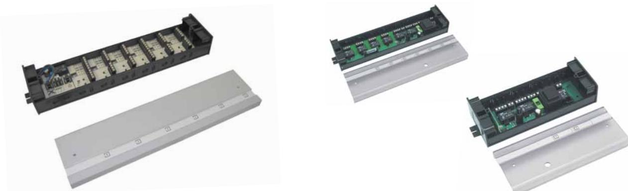
The Basic terminal block for heating and cooling with a pumping module in a 230V and 24V version allows to connect thermostats and actuators at one place in an installation cabinet above a manifold. Maximally you can connect 6 thermostats and 6 actuators.
