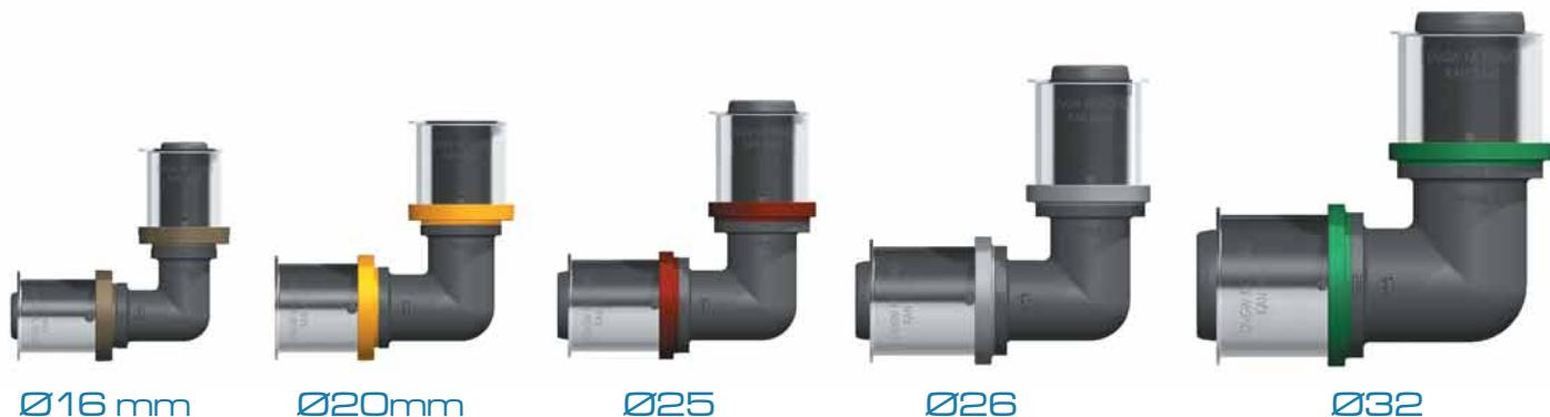
Such solution makes work more efficient both in the warehouse and in the construction site where it is difficult to identify fitting diameter (ex. lack of light). Regardless of the color identification, each nozzle is marked with diameter of connected pipes. Dimensions of connected pipes (outer diameter x wall thickness) are also marked on the steel sleeve.
