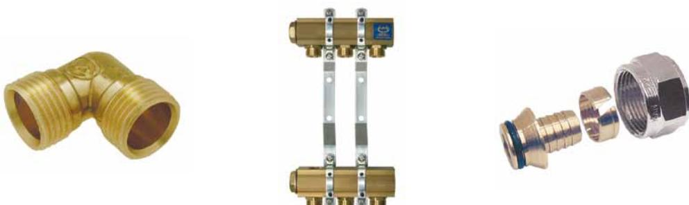
Eurocone adapters are characteristic for a sealing on the cone and an O-ring between body and a fitting. This kind of joints is self-sealing and no additional sealing element like a PTFE tape or tow shall be used. Locate such connections at generally accessible places.
