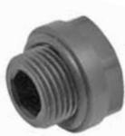
It may be repeatedly use (has O-Ring seal) and should be used for all **KAN-therm** wallplate elbows and wallplate tees. Plastic short plug is used only to make the pressure test and it cannot be use to blank off the installation permanently.
