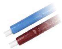
**KAN-therm** multilayer pipe PE-RT/AI/PE-HD Multi Universal designed for central heating, hot and cold water systems as well as for underfloor heating systems; operating pressure max. 10 bar - in 6 mm thermal insulation
