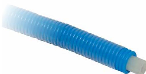
Due to such a design between a PE-Xc pipe and a protective PE-pipe there is a layer of air, which reduces the amount of heat given up. PEX70 pipes can be used to lay a floor heating connected to a radiator installation, where the supply water temperature does not exceed 70°C. PEX70 pipes are delivered in coils.
