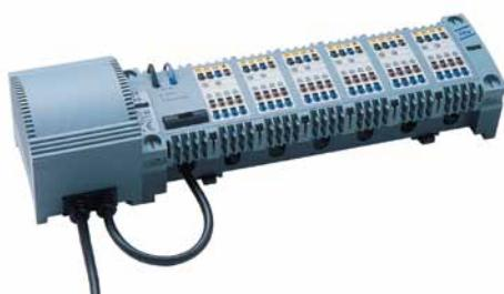
The Premium terminal block - version 230V and 24V - allows to connect thermostats and actuators at one place (e.g. in a box above a manifold). At the most you can connect 6 thermostats and 14 actuators. A strip can be extended by additional extension modules (e.g. an actuator extension module or a thermostat extension module etc.).
