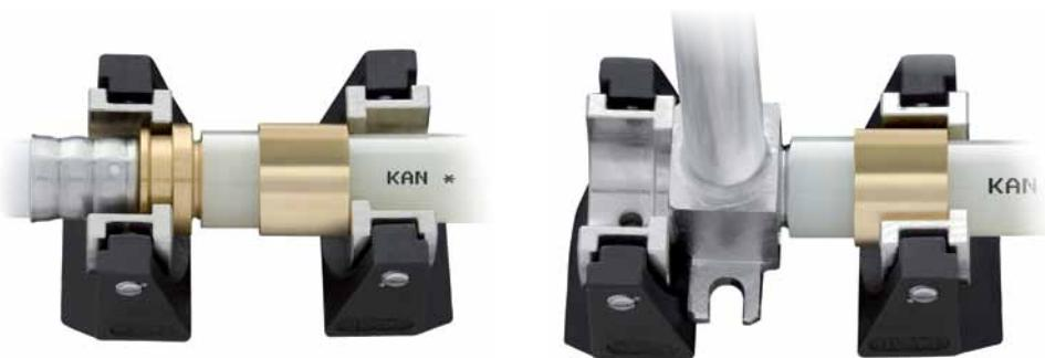
6. For tees (stub pipes at branches) Ø14, 18, 25 mm at the side of fittings use nickel-plated shaped inserts marked: P8465, P8463, P8468, P8464. At the ring side use nickel-plated straight inserts.
