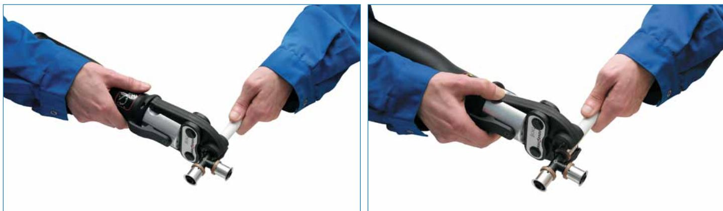
5. Start the press drive and make the connection. The process of pressing lasts till the jaws close fully.
