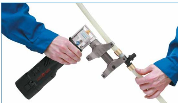
4. Insert the fitting into a pipe up to the last bead on the fitting.
