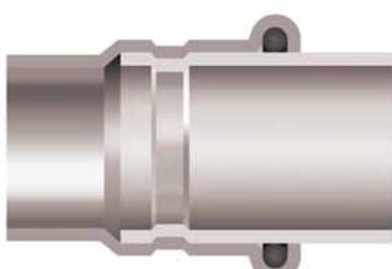
**Pic. 5** Press conection before and after press
