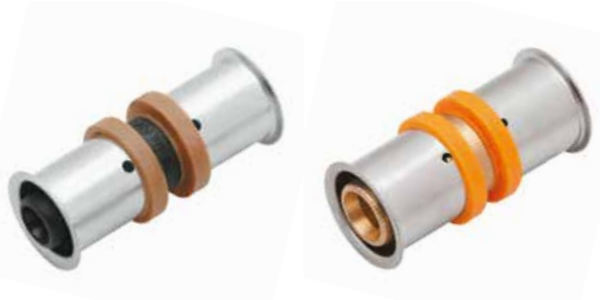
Slika 50. KAN-therm ultraPRESS spojnica za PERTAL, PEXC, PERT i blueFLOOR PERT cevi 14mm × 2 mm, 16mm × 2 mm, 20mm × 2 mm, 25mm × 2,5 mm.
